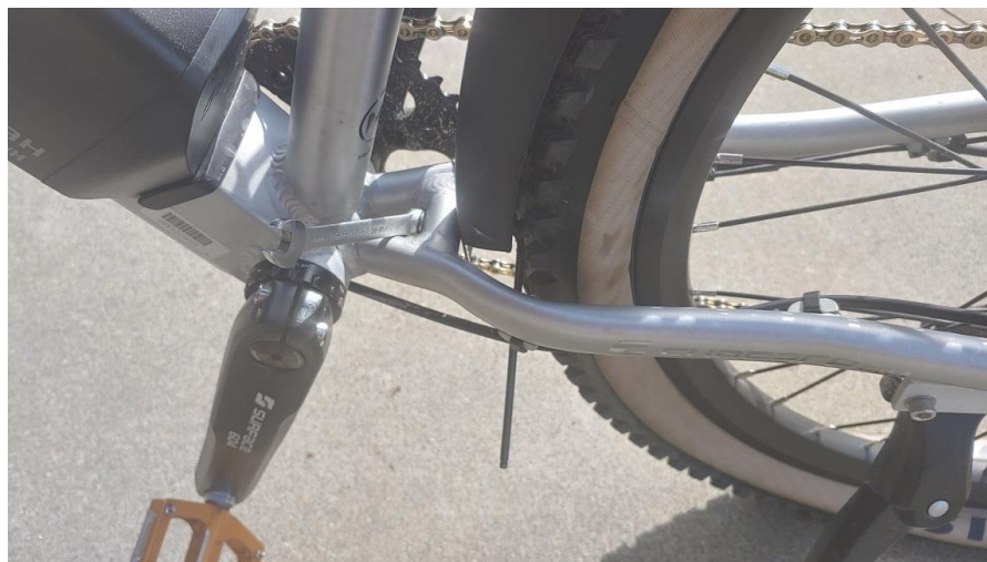
Deflating the rear tire makes it easier to install the lower nut and bolt.
