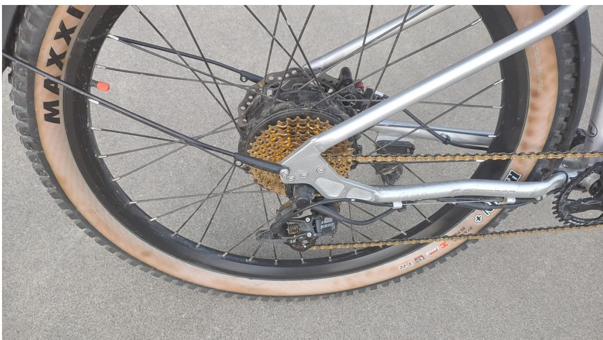
Deflating the rear tire makes it easier to install the lower nut and bolt.
